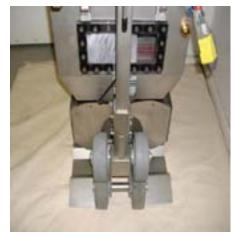
Using the (2) long 36" bungee straps provided, attach to one of the holes on the front of the Caddy (opposite the wheels) and hook the top end onto the hose arm. Repeat on the opposite hole and arm for the second strap. The bungees should be crossed for added stability.
