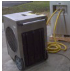
29: Fancoil Connected to HD308 Unit
