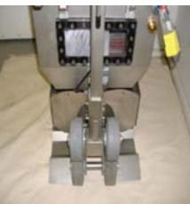
Using the (2) long 36" bungee straps provided, attach to one of the holes on the front of the Caddy (opposite the wheels) and hook the top end onto the hose arm. Repeat on the opposite hole and arm for the second strap. The bungees should be crossed for added stability.
