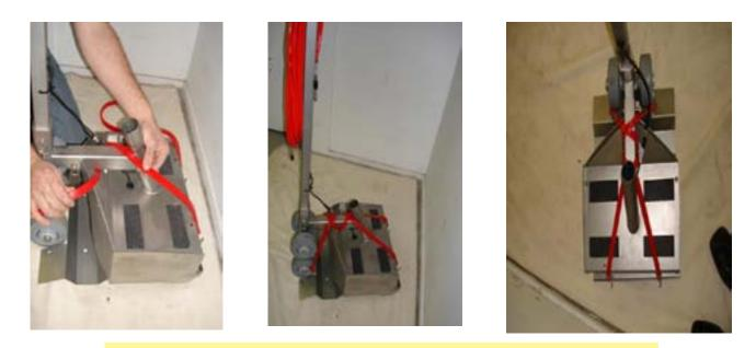
**NOTICE:** The longer straps are used for this, and have to be wrapped once around the stem. The short strap is not used in this scenario.
