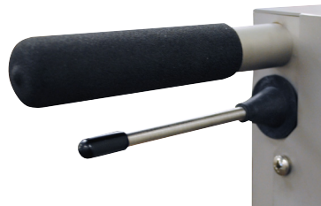
Figure 4: Compress the movement handle when ready to begin extraction.
