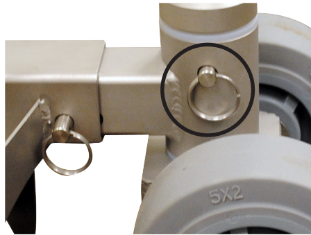
Figure 2: Remove the hitch pin to steer the Hydro-X during extraction
