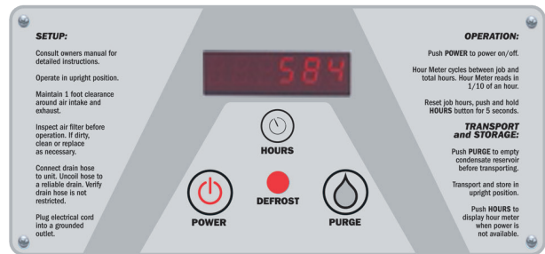
Phoenix R150 50Hz control board.
