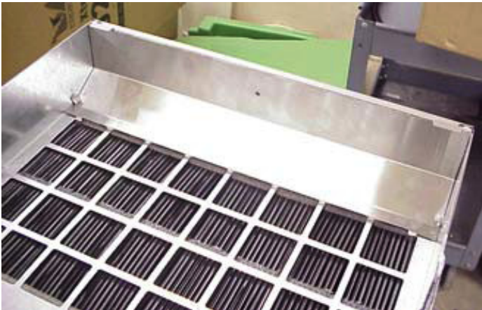
Figure 1: Bracket installed in Phoenix HT using existing fasteners. Note tabs bent down between plastic heat exchanger panels. 200 MAX installation is similar
